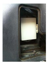
Note that the factory oem cable connectors need to be routed so they plug into the side of the unit unlike the factory unit where they come into the bottom.
